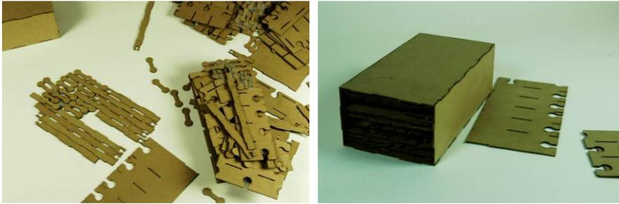
**Figure 4 Left, photo of dog bones, studs, and wall panels with notches for dog bone connections cut of 1/16" cardboard stock simulating 3/4" plywood sheets
