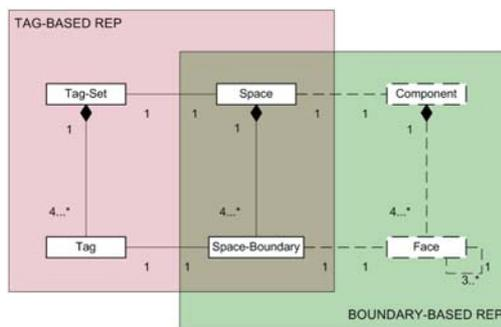
**Figure 1 Tag-based and boundary-based space representations (dotted lines indicate derivation by spatial reasoning)**
