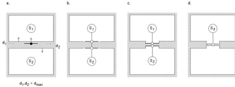
**Figure 4 Opening representations and space connectivity. a. matching of opening-tags and space-boundary-faces; b. opening-faces co-planar with space-boundary-faces. c. recessed opening-faces; d. disjoint opening-solid filling a hole connecting two space-components.**
