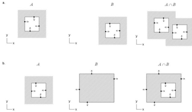
**Figure 3 Merge of bounded and semi-bounded components by boolean intersection. a. Merge of two space-components; b. Merge of an envelope-component and a space component**
