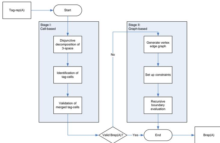
**Figure 2** Flow diagram of the procedure converting a tag-rep(A) to a Brep(A)
