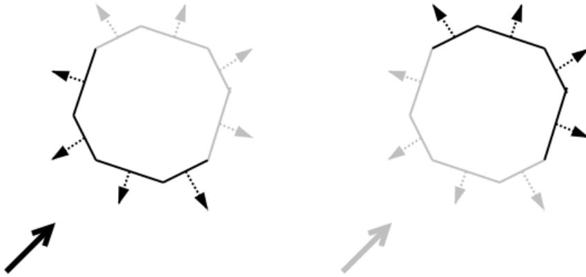
**Figure 2 Normal (left) and inverted perspective (right) display modes. The long arrow indicates the viewing direction. Black edges represent faces which are drawn; grey edges represent faces which are not drawn**
