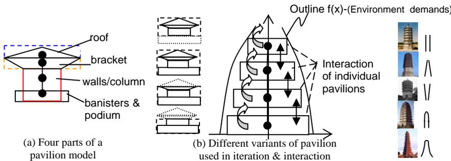
**Figure 4 Diagrams for the Structural and Interaction Models**
