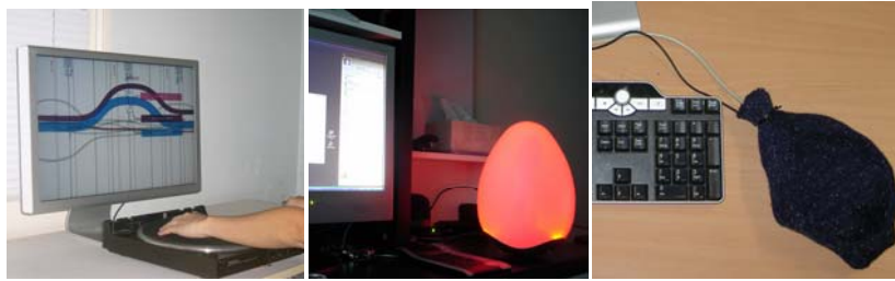
Figure 6. infodevice course results. Left: Data Scratching, exploring time-varying data by Video Jockeying (Author: Sheryl Soo), Middle: Dino, an egg-shaped device that moves in reaction to emotions during online chat conversations (Author: James Kim), Right: FeelMouse, a computer mouse that alters temperature depending on textual emotions (Author: Irene Chen).
