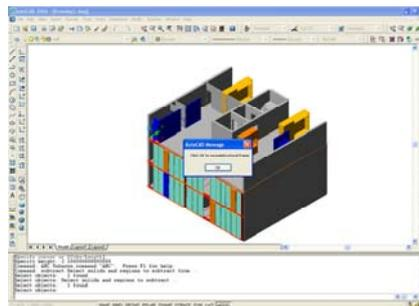
*Figure 6.* A 3-dimensional model of the evolving design is displayed to facilitate assessment and decision-making.
