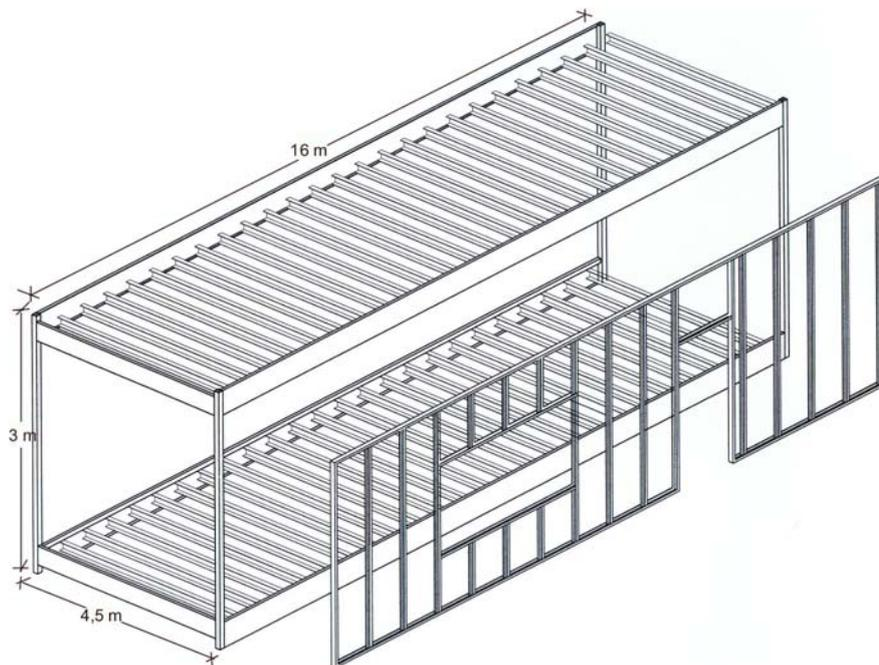
*Figure 4.* Structural and framing system from the Kingspan building system. Typical prefabricated grid with maximum dimensions.
