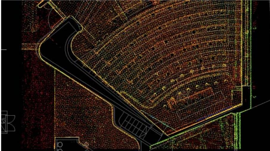
*Figure 2.* Example of inventory data from HUT's Department of Architecture building. Integrating the architect's original drawings (Alvar Aalto, 1961), digital inventory drawings (1994) and contemporary 3D-laser scanning data (2006).
