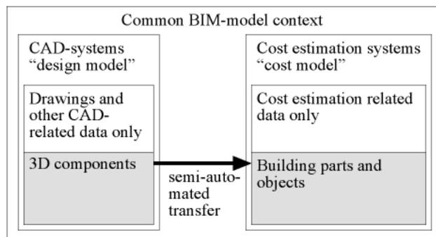
Figure 3. Diagram of CAD and cost-estimation data contents in relation to BIM.
