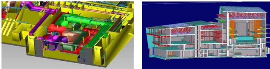
*Figure 3.* Left: view of the common model. Right: Visualization of structural systems, with the façade “reference shells”. (Courtesy: Rambøll Danmark A/S).
