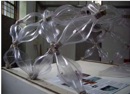
*Figure 1.* One of the structural prototypes (Lattice grid), 1:2 scale mock-up.
