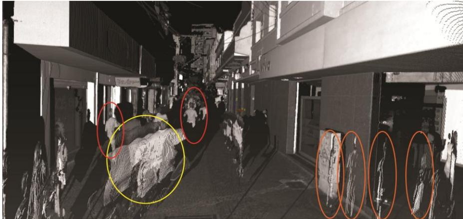
**Fig. 5.** Different recordings of people in a point cloud (position B, high resolution).
