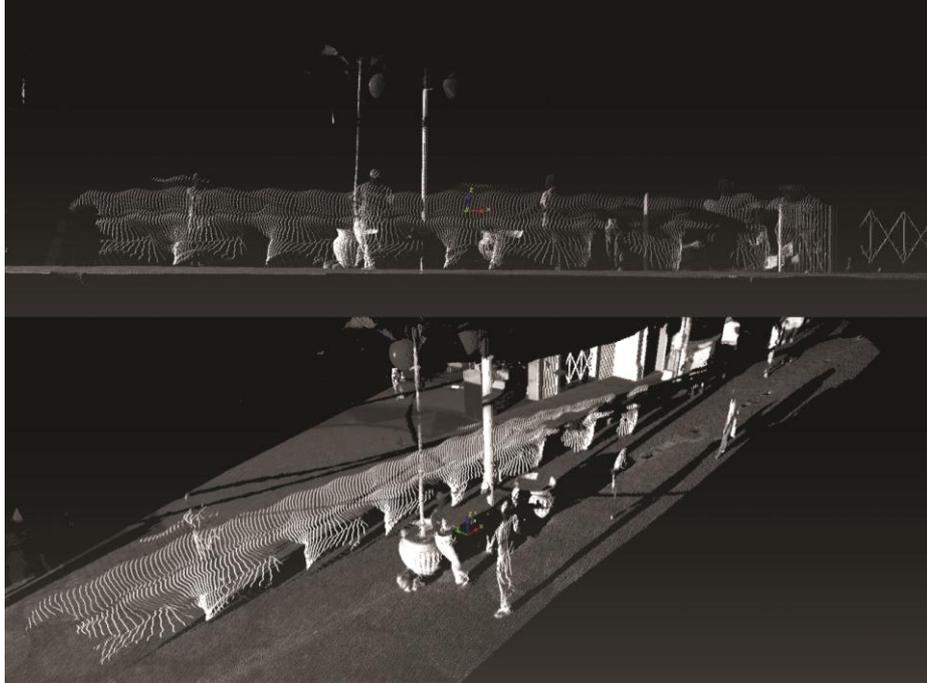
**Fig. 4.** Recording of a pedestrian's path walking in the same direction as that of the laser scanner rotation (clockwise) as compared to people in a static position (position A, high resolution).
