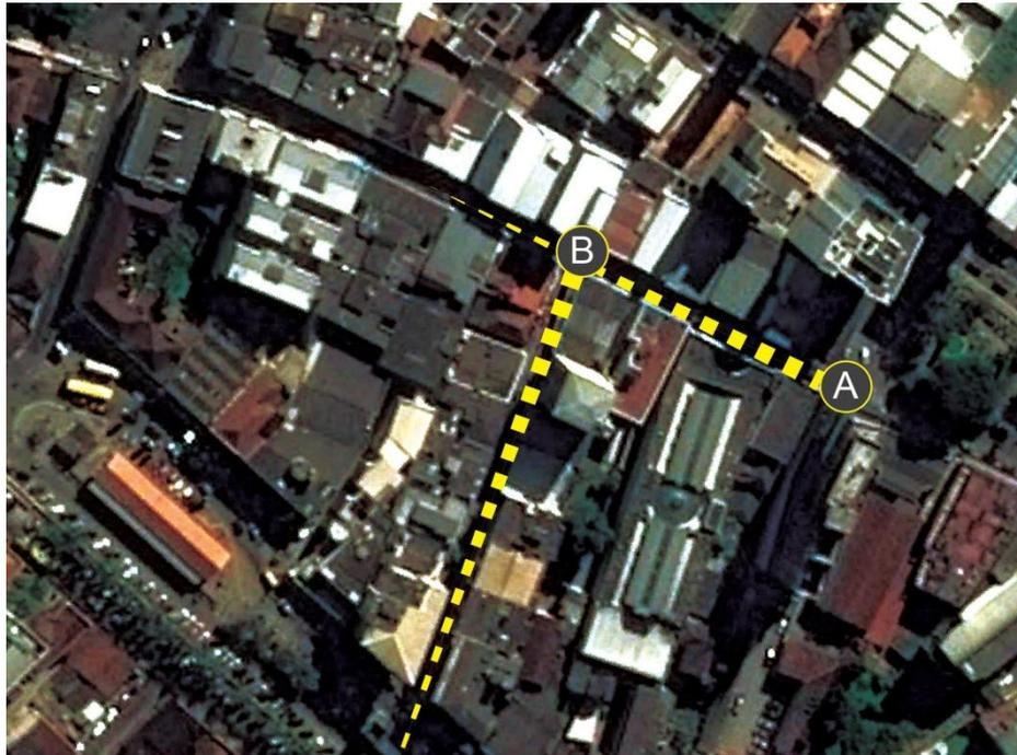
**Fig. 1** Axes indicate road and positions A and B of laser scanner during experiment.
