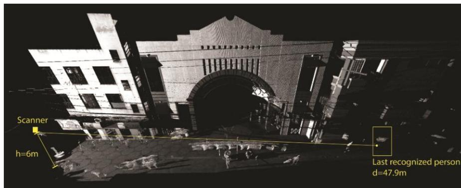
**Fig. 2** Analysis of patterns of points enables recognition of people. Image of point cloud showing the farthest person recognized at high mode at position A.
