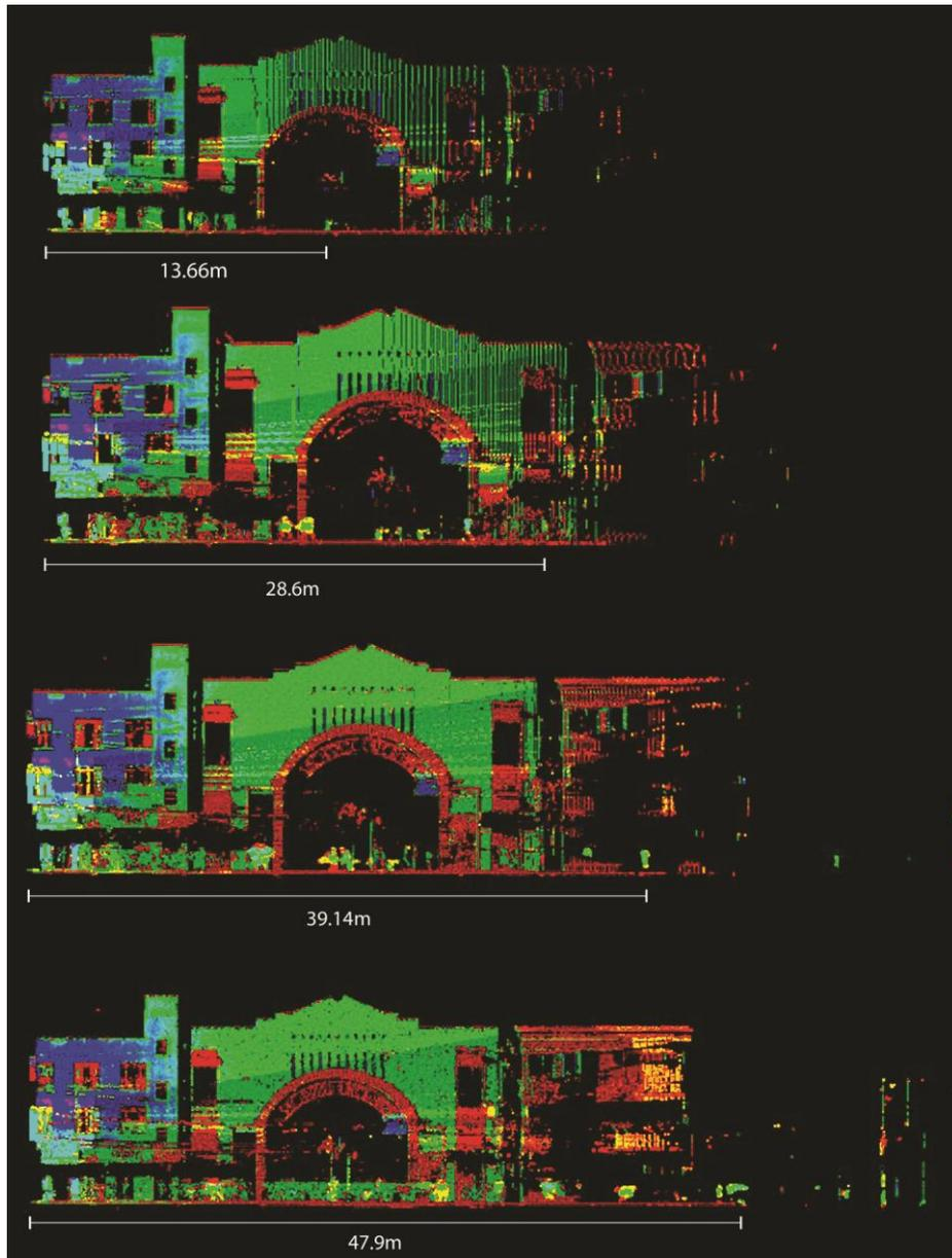
**Fig. 3** Maximum recognition distance at standard resolutions preview, low, middle, and high at position A.
