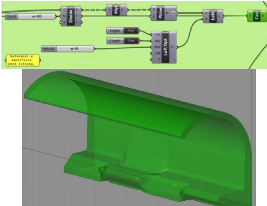
**Fig. 10.**Lofting control algorithm and virtual model
