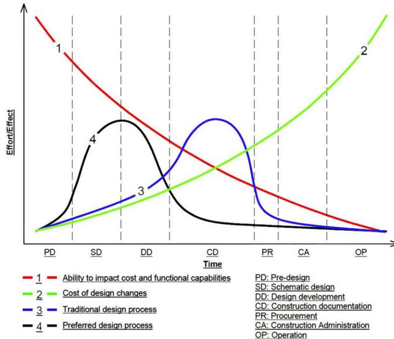
Fig. 1. Design approach and effect comparison. [4]
