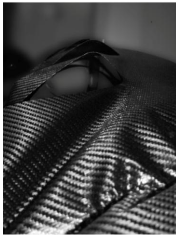
Fig. 3 - cuts and pleats for surface articulation. Pre-preg Carbon 0/90 Twill, 600 gr/m 2
