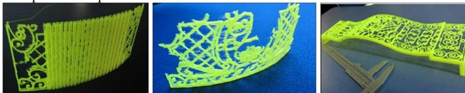
**Fig. 7.** Problems faced in 3D printing the balcony [8].
