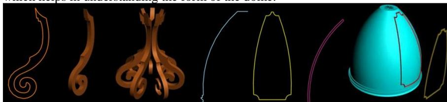
**Fig. 3.** Decomposition and recomposition of the dome.
