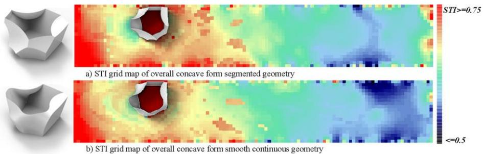
Fig. 6. Odeon simulation comparison, Set II
