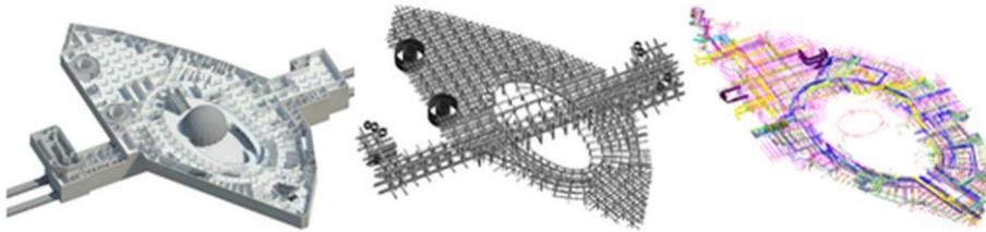
**Fig. 7.** The figure on the left shows the model from architecture department; the figure in the middle shows the structure design; the figure on the right shows the models of pipes, cables and instrument developed by the equipment design department
