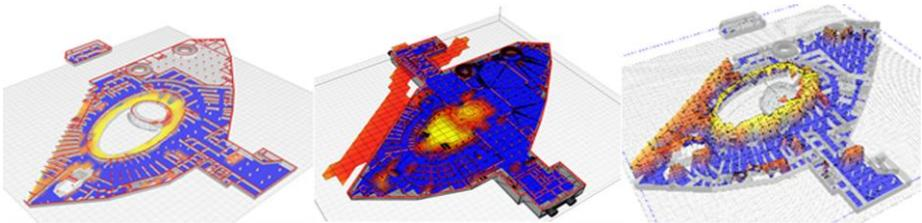
**Fig. 4.** On the left, the image is the illuminance analysis of Basement Level 1. In the middle, the image shows the analysis of Basement Level 2; on the right, the image shows the 3D display of the illuminance value of the Basement Level 1
