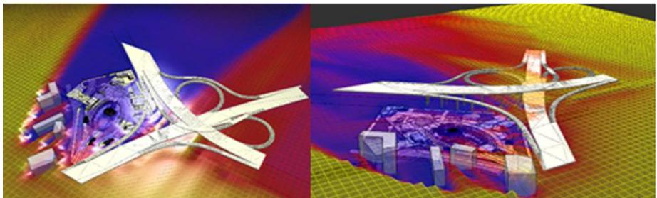
**Fig. 5.** The images illustrate the wind environment analysis based on BIM
