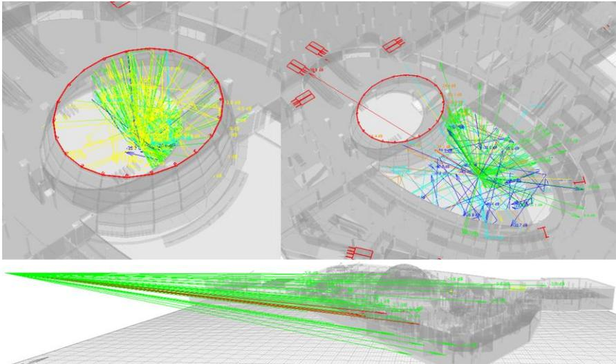
**Fig. 6.** The models illustrate the acoustic performance analysis: Top-left shows the reverberation simulation in the glass dome; top-right shows the reverberation simulation in the atrium, and the bottom figure shows the noise analysis
