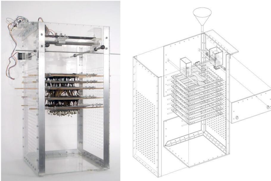
**Fig.1.** Motion Capture 3D Printer and Axonometric Drawing
