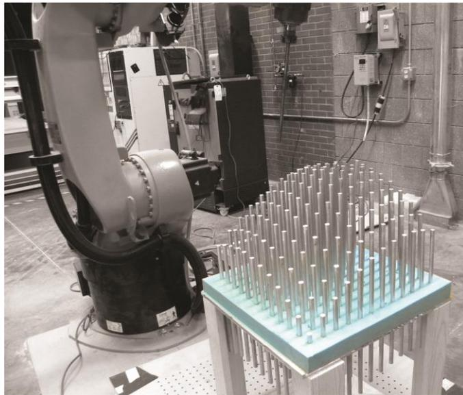
**Fig.6.** Reconfigurable pin-mold
