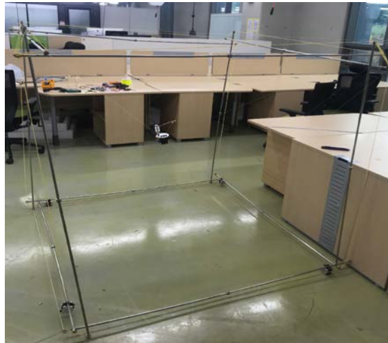
Fig. 1. Eight-strut tensegrity structure built in this project. An extruder head is located at the center of the structure. Stepper motors are installed on bottom struts.
