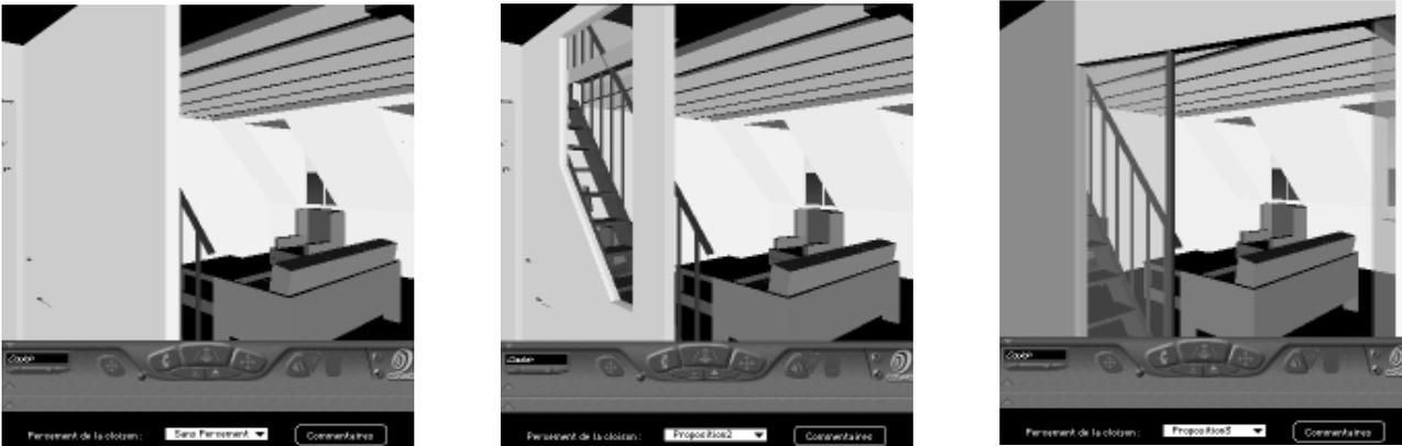
Figure 12. Architect's alternatives to answer the owner's question about daylighting in the corridor. Original design proposal (left), with a hole (middle), with a glass door (right).
