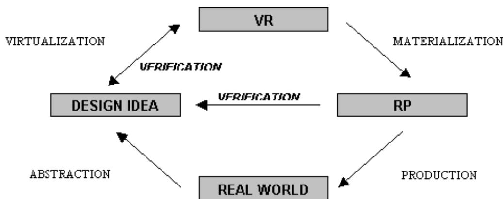
Fig. 2: the design process after the adoption of VR and RP technique
