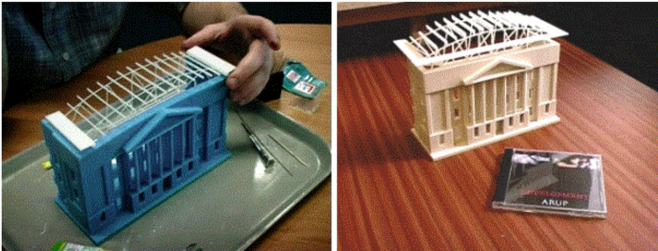
Fig. 1: two models made with RP technology: the first design solution (left) of the truss was changed and in the second project (right) a new different material was also used for the walls.
