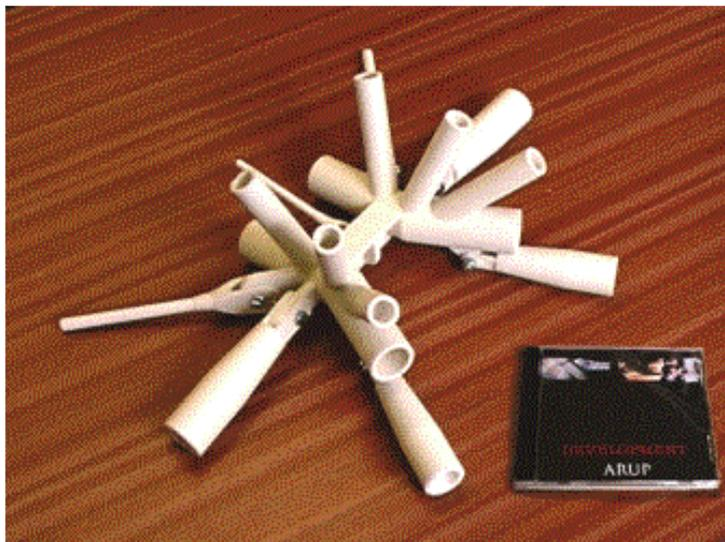
Fig. 4: the joint built with the 3D printer
