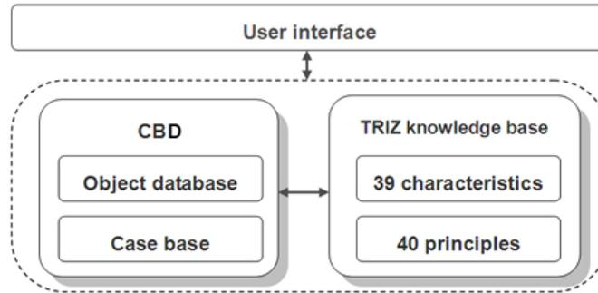
Figure 10. System architecture.
