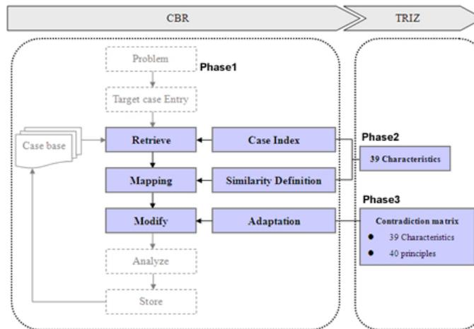
Figure 9. Integrate TRIZ into CBR design system.
