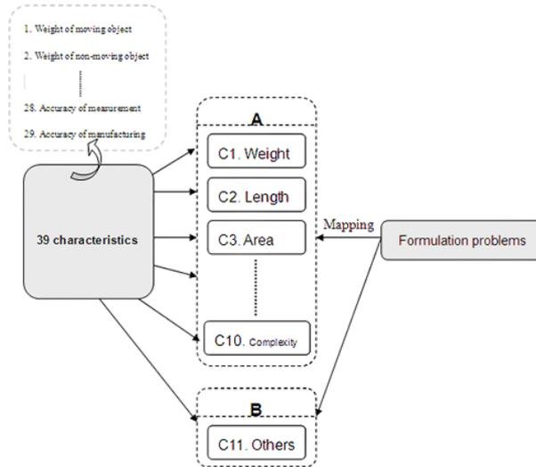
Figure 8. Design problem mapped into grouping of 39 characteristics.
