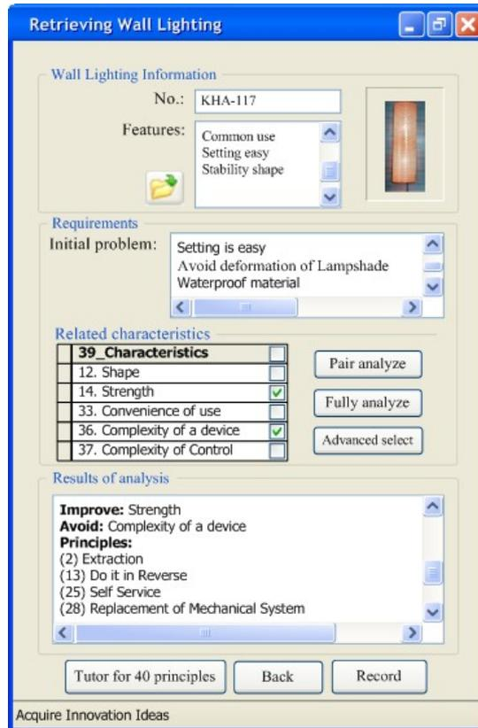
Figure 14. GUI of innovation principles by contradiction matrix.
