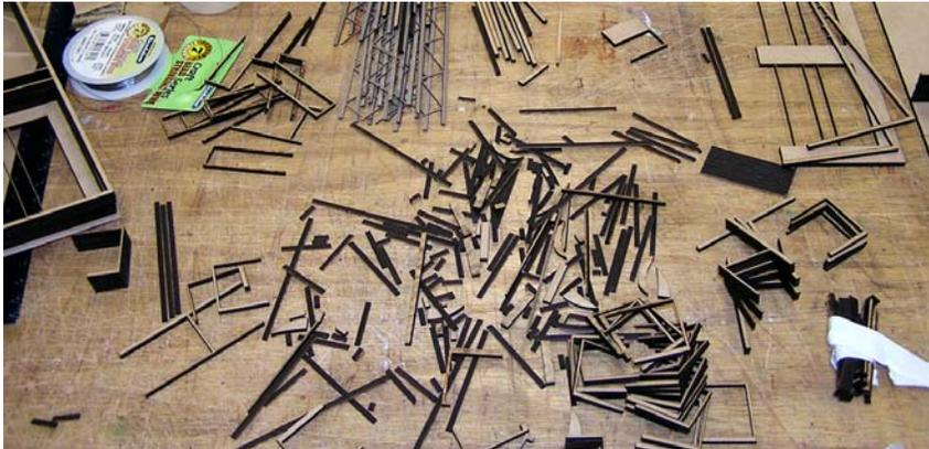
Figure 17. *Ready-to-be-assembled model parts from the laser cutter*
