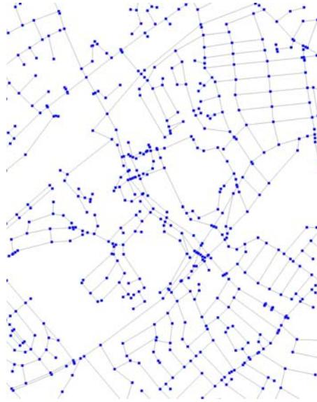
Figure 7. The converted ITN with straight segments and reduced number of nodes.
