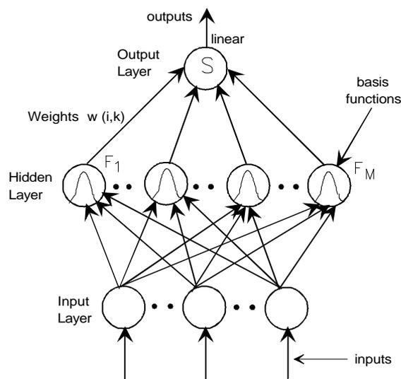
Fig.4: Architecture of a basic radial-basis function network having only one output
