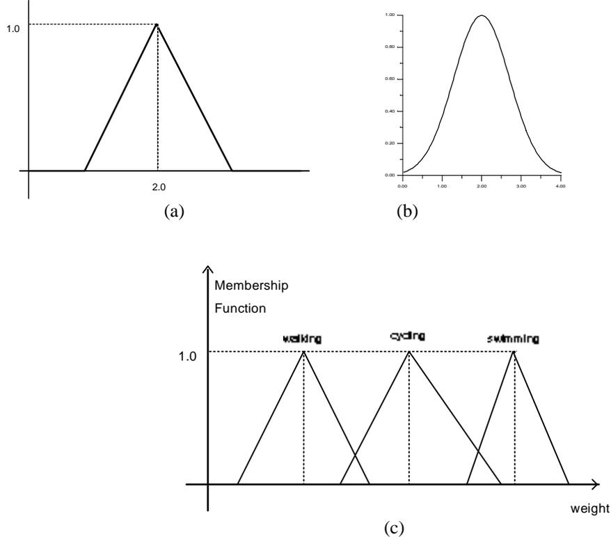
Figure 1: Examples of membership functions for characterizing fuzzy sets in different contexts (a) triangle shaped (b) gaussian shaped (c) Fuzzy sets of weights representing difference in sports
