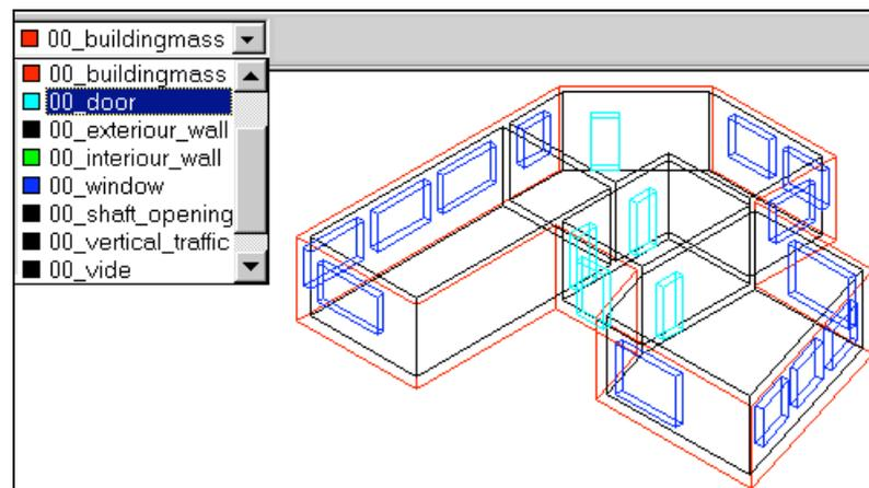
Figure 2: **Modularization of geometry**
