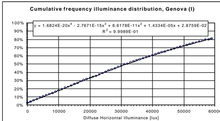
Figure 1: Example of polynomial function used to calculate daylighting autonomy, (Metetest 2002)
