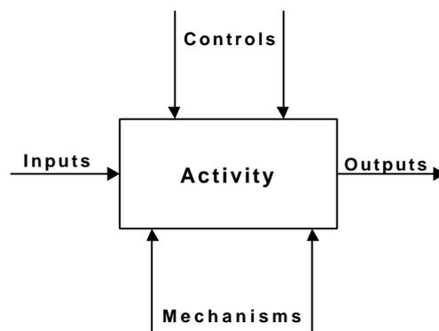
Figure 1: IDEFØ Function Box and Interface Arrows (KBSI 2000)
