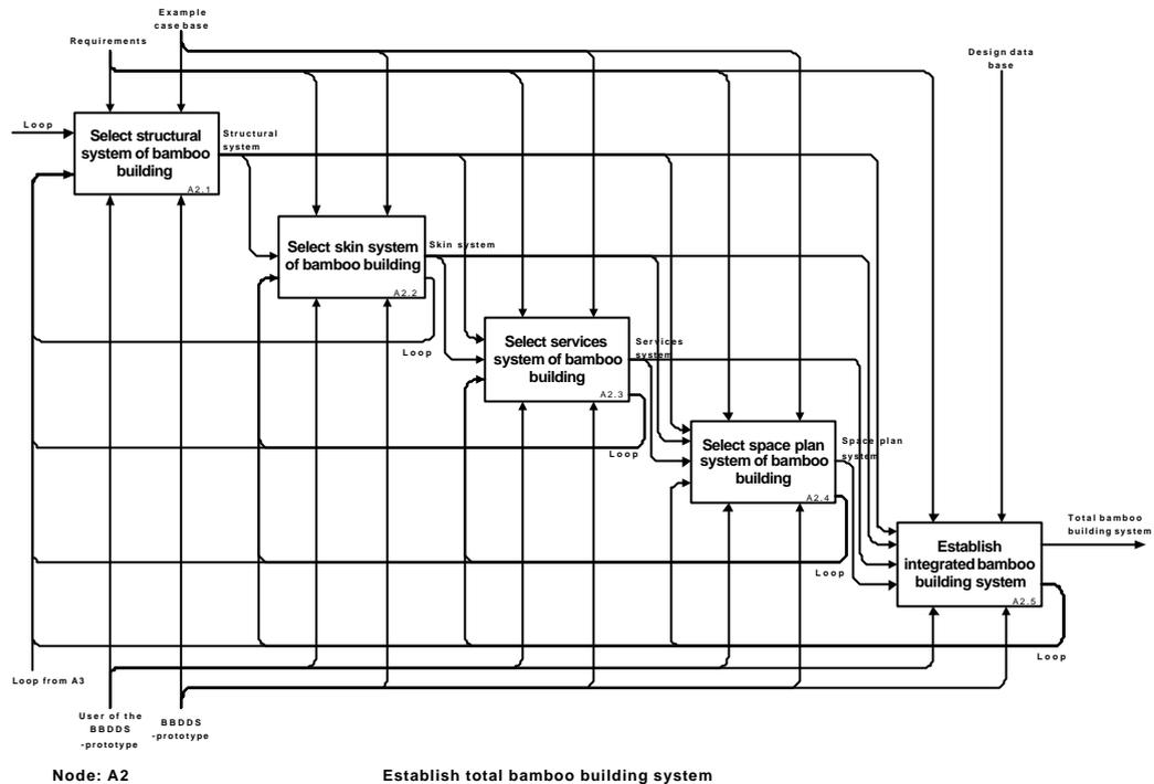
Figure 2: An IDEFÆ Scheme for Bamboo Building Design
