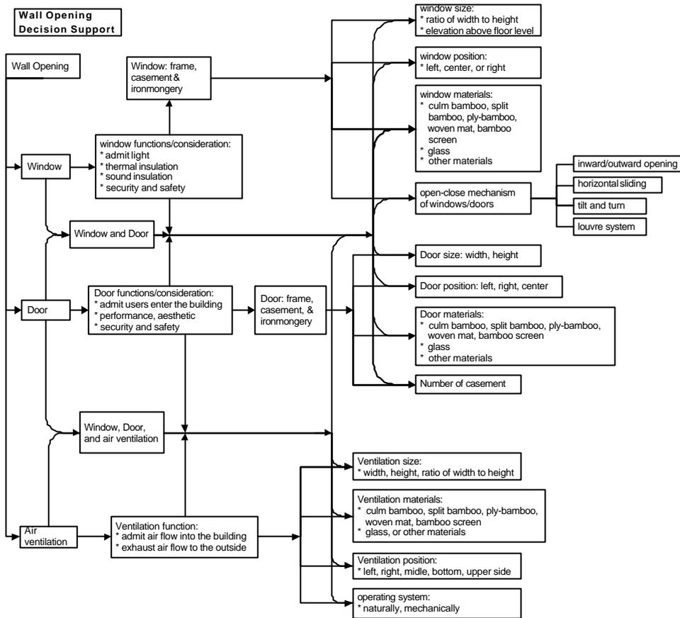
Figure 5: Decision support for wall openings design process
