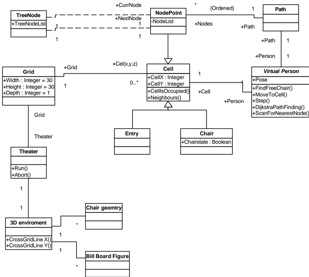
Figure 5: Class diagram simulation system
