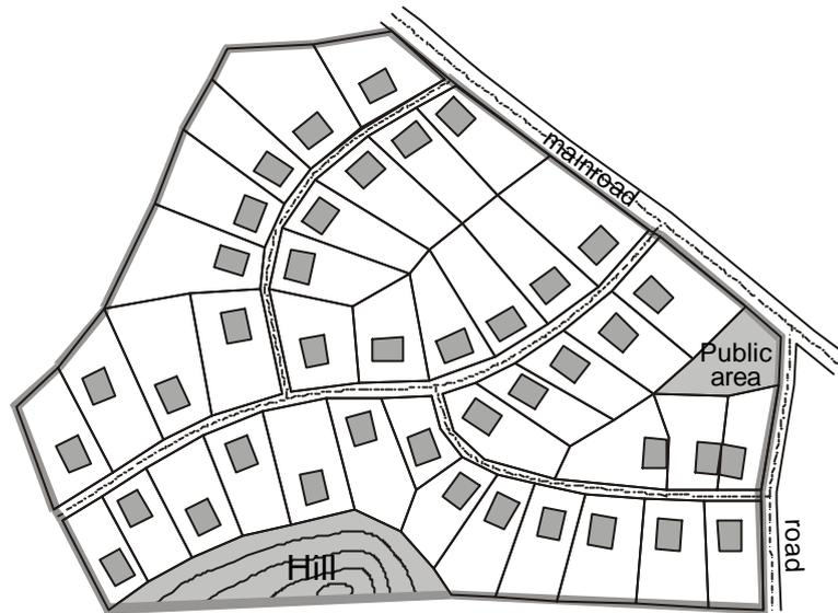
Figure 7: **Combining road access with site partitioning**
