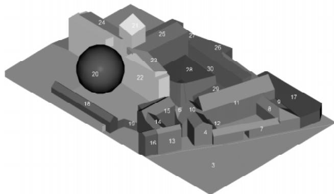
Figure 7. Phase 1 and 2, modelling the terrain and (both existing and new) building blocks of the masterplan. The numbers on the geometrical entities refer to the primary key of the corresponding *ELEMENT* in the Access database. The main building block and tower (in lighter colour) will be further elaborated in later design stages.
