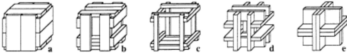
Although only the proportions of the originally square section of the sticks defining the edges are changed, resulting configurations are quite different from each other. 9.a represents the cube as a box, where 9.e represents the cube as a node, both being built up by elements of the same size which are no more sticks but boards.
