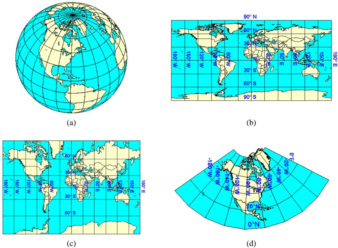
**Figure 3:** Examples of geodetic and projective coordinate systems. (a) Orthographic projection, used for perspective views of the earth, moon, and other planets, (b) latitude/longitude graticule, used to locate points on the earth's surface via a grid of meridians and parallels, (c) Mercator projection, used for navigation or maps of equatorial regions, (d) Lambert Conformal Conic, used by USGS for topographic maps. (Images adapted from Dana<sup>10</sup>. Reproduced with permission.)
