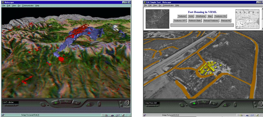
**Figure 2:** Two examples showing the embedding of georeferenced objects. The image on the left shows a weather simulation over the Colorado Rockies, while the image on the right shows an airstrip with georeferenced 3-D geometry for roads (orange) and buildings (yellow). These and other terrain datasets can be browsed from <http://www.ai.sri.com/VRMLSets>.
