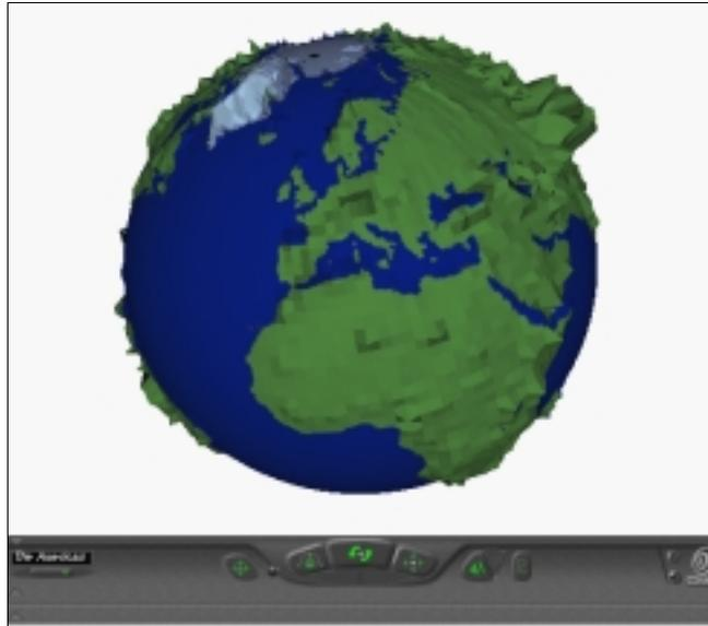
**Figure 4:** Illustrating the use of the GeoElevationGrid node to insert latitude/longitude coordinates directly in a VRML file. These coordinates are transparently transformed to geocentric coordinates to produce an ellipsoidal model of the earth. We have exaggerated all heights by a factor of 200 to highlight highly mountainous regions such as Greenland and the Himalaya.
