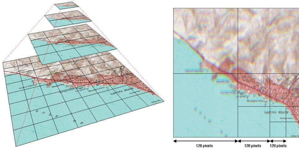
**Figure 1:** Illustrating a tiled pyramid representation. The left image shows four different resolutions of a digital map where each level has been segmented into a regular grid of tiles. The right image demonstrates the use of a quad-tree technique to alter the resolution of an image in different regions.
