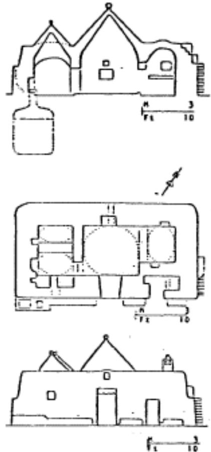
Fig. 4 Longitudinal cross section, plan and south elevation of the "Trullo" studied.
