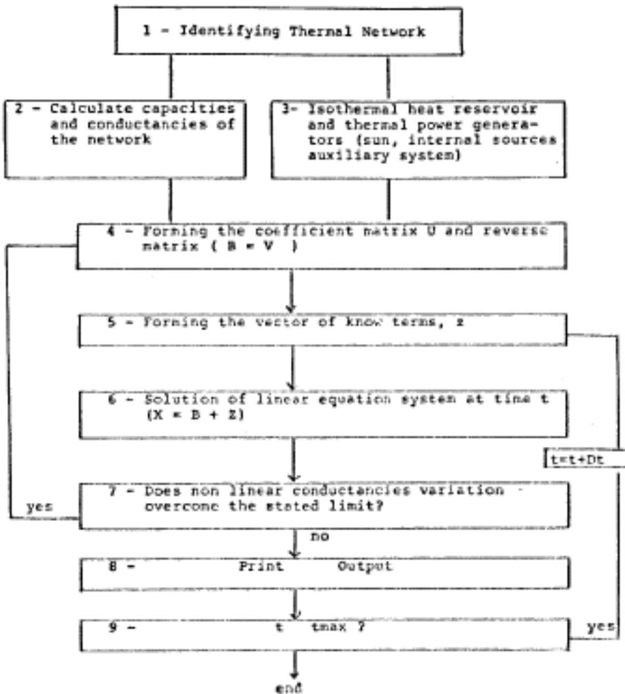
Fig. 1 - Block diagram of BEETA simulation code
