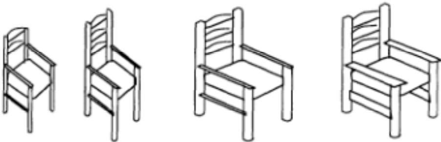
**Figure 14.** Stylistic transformation of chairs dealing with both overall proportions and proportions of parts. The left is a scandinavian style, which is re-scaled into the ones to the right, becoming one with mission style. The number of back slats was also reduced.
