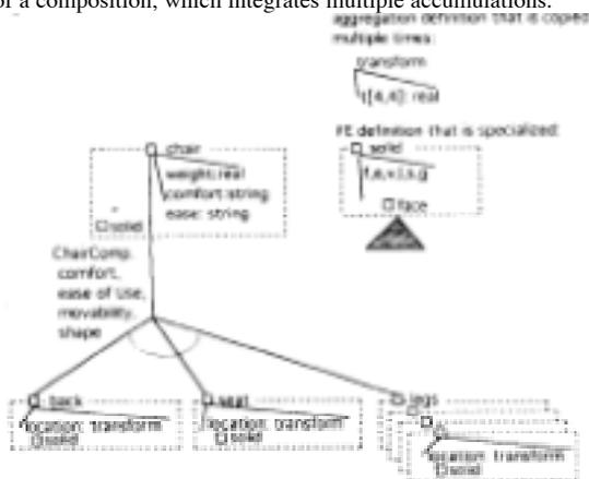
Figure 6. The simple conceptual definition of a chair, based on the dictionary definition.
