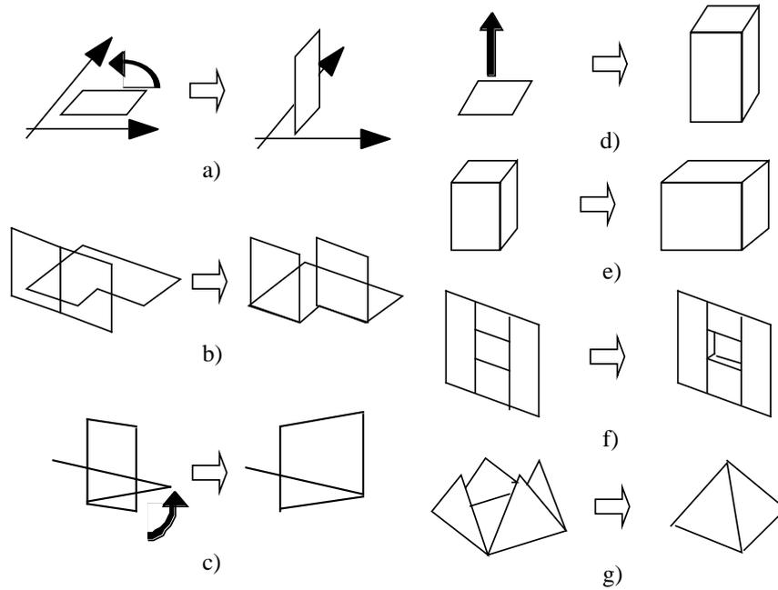
Figure 1. Seven typical operations in architectural modeling.
