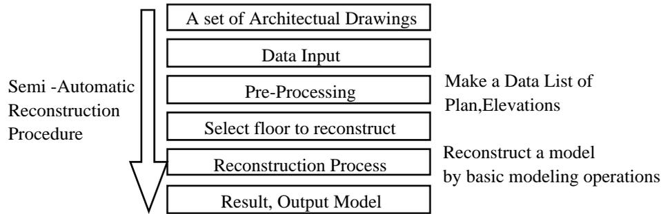
Fig.2. Operation flow of reconstruction processing
