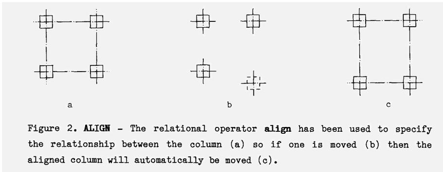
Figure 2. **ALIGN** - The relational operator **align** has been used to specify the relationship between the column (a) so if one is moved (b) then the aligned column will automatically be moved (c).
