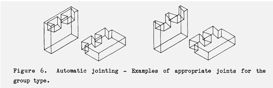
Figure 6. Automatic jointing - Examples of appropriate joints for the group type.
