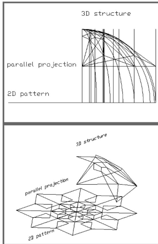
**Figure 5 :** parallel projection shown on an example (1/4 projection)
