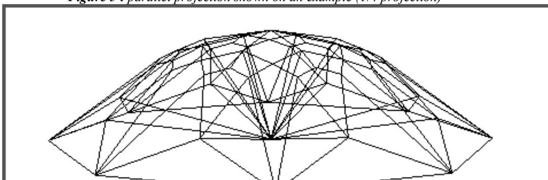
*Figure 6 : result of parallel projection*
