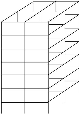
Figure 9. Building structure with horizontal lateral bracing added.
