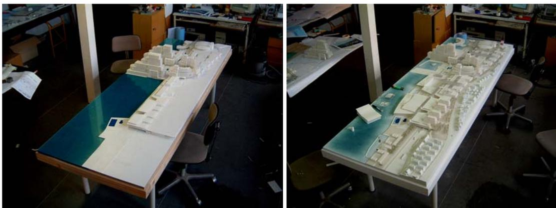
polyurethane-based material with good strength and toughness, which is easily mechanically elaborated. A representative of this material are Sika-Block – model plates – which are produced in the thickness from 50 mm up with various physical properties. Its characteristic property is homogeneous, fine-grained structure of material with slight moisture-absorption. The strength of its edges during abrasion is very good.
