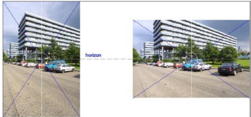
**Figure 09:** The middle of the picture is marked by two diagonals: it shows the height of the untilt camera and marks the horizon
