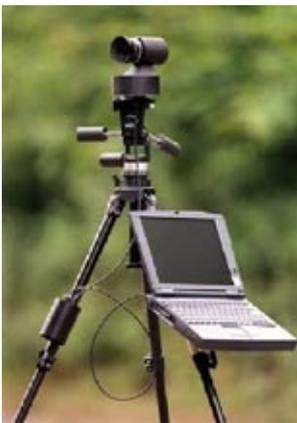
**Figure 15:** Highly professional camera equipment: the digital scanner panorama camera SPHERON, directly connected to a notebook.
