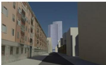
Figure 11: Shadows' simulation using the 1:1000 scale maquette in the heliodon: future condition
