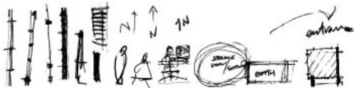
*Figure 2.* Designers share drawing conventions: They used lines, arrows, hatches and simple geometric shapes to compose symbols for architectural objects such as walls, windows and stairs. Words are used to indicate directions and functional spaces.
