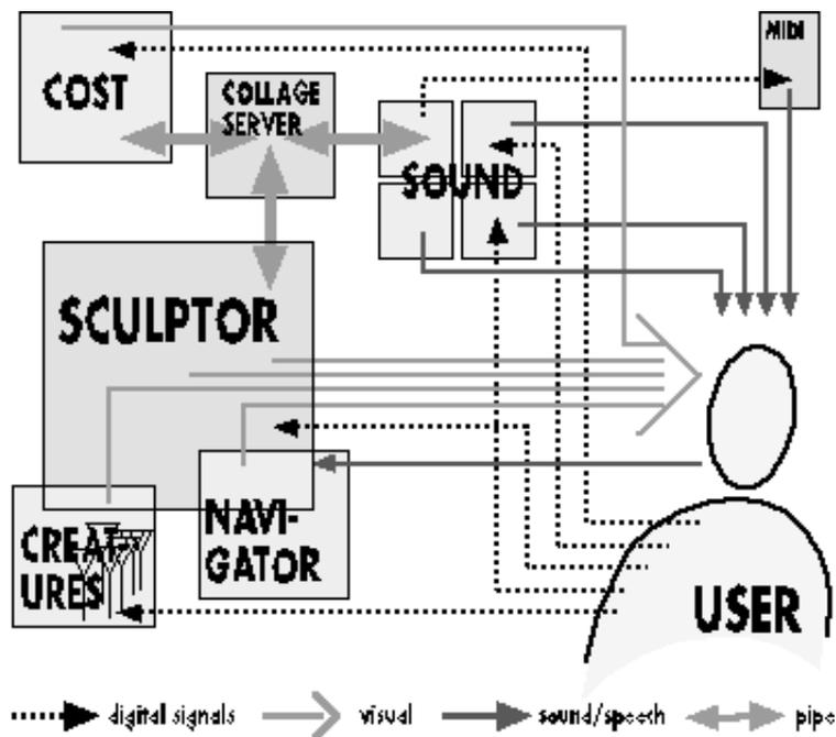
In the current state of the project, the described properties are implemented in prototypical ways. The core of the design environment is comprised of the 3D-modelling tool "Sculptor" (Kurmman 1995), that allows intuitive and interactive modification of intelligent objects. The designer can interact directly with Sculptor or employ different kinds of agents for further help. Figure 2 shows the various parts of the environment and the channels for interaction.
