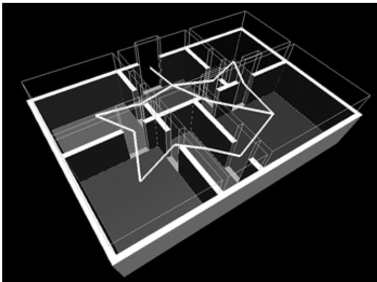
The Navigator Agent generates the graph of the movement after analysing the scene. It calculates the possible path to its goal, and it considers the constraints at hand, such as no-collision and moving-up and down stairs. All these constraints are integrated into the modular program Sculptor.
