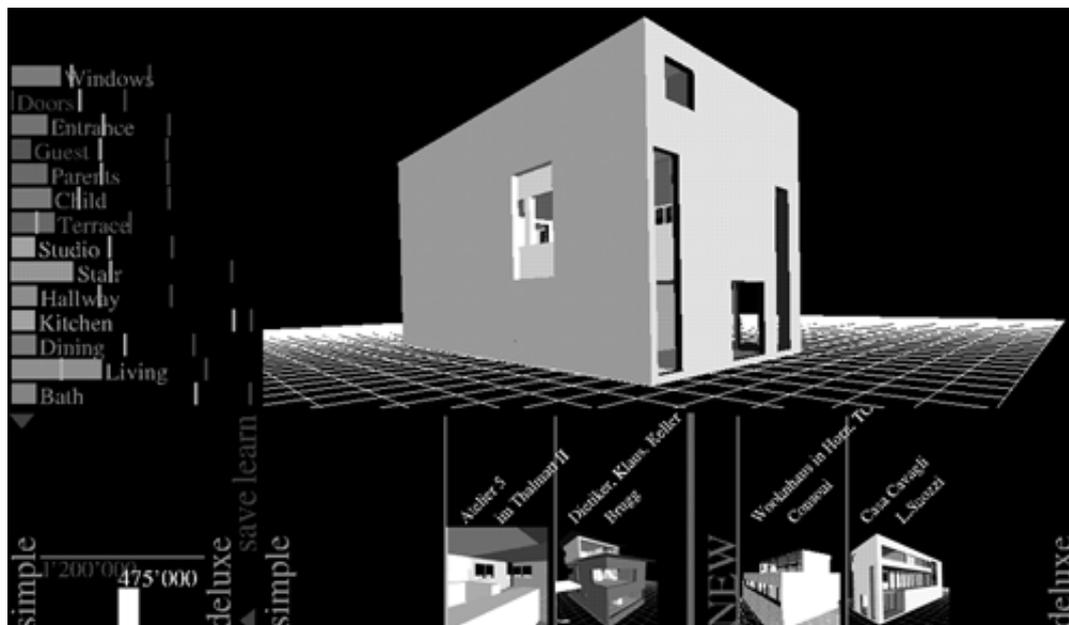
The Cost Agent has additional interfaces for a space by space cost analysis and to a database of built projects of which the costs are known. These are ordered according to their deluxe level. For new projects, the deluxe level can be indicated within the sequence.
