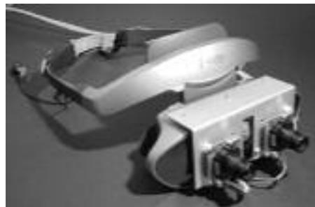
Figure 1. Cy-Visor with attached PAL cameras
