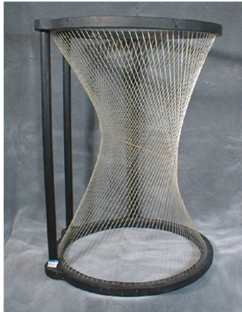
Figures 1, 2 The 'Hyperboloid of one sheet' is a type of ruled surface used by Gaudi in the design of the Sagrada Familia; rendering of a nave window from the Sagrada Familia: it has resulted from Boolean subtractions of ruled surfaces from a notional solid (Burry 2004)
