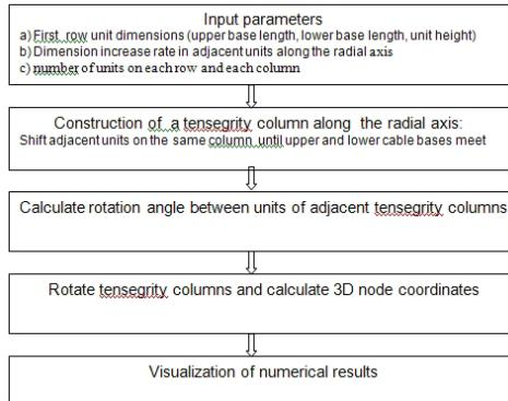
Similarly the scheme in Figure 5 compares the process to be followed for the geometric construction of a 6 unit vaulted configuration, to the required process for the generation of a six unit helical configuration composed of sets of self-similar but not identical units.
