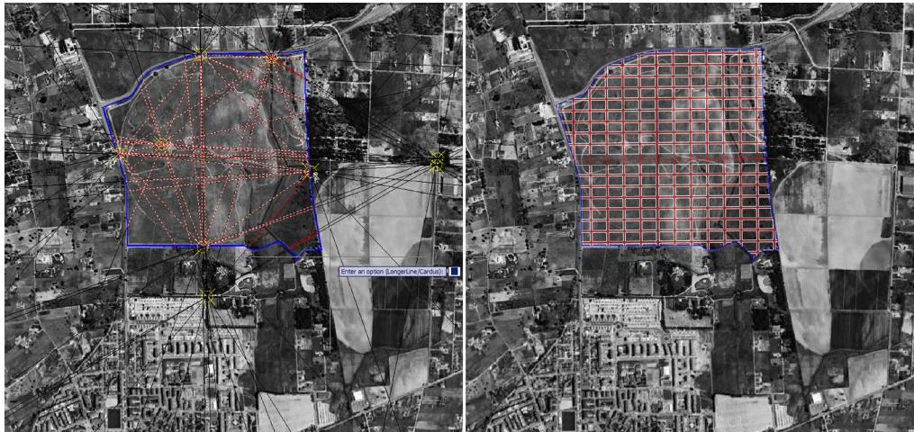
Figure 1 - Grid generation: 1- Selection of points defining reference points; 2- Generation of the grid.
