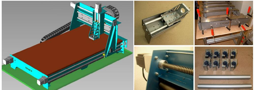
to combine low weight with high torsional stiffness. The precision in its construction is mandatory for the resulting tolerance and precision of the whole machine. To reduce costs we choose solid aluminum 10 x 10 mm, which can be delivered cut to size. Furthermore, additional holes for fastening e.g. energy chains, distribution boxes, dust shields, exhaust mountings etc. are easily drilled.
