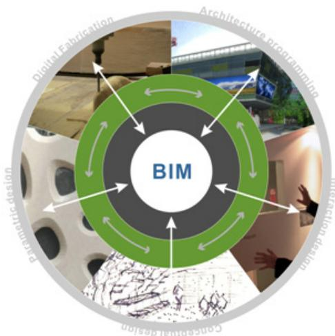
We develop a design framework using BIM to integrate varied design process. The BIM-centered design framework includes five parts: architectural programming, conceptual design, parametric design, digital fabrication, and interaction design.
