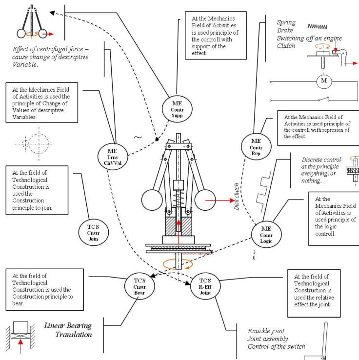
The design process continues by the input of these descriptions (x1, x2, x3) into the CRDP software and generation of suggestions of a new conceptual solution. The suggestions have a form of sign chains.
